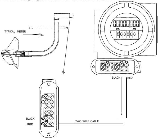
The positions of the wires in the condulets is not important. The black wires should be connected together, and the red wires should be connected together.
