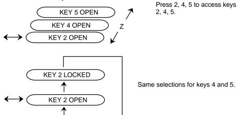
The Totalizer and Ratemeter HI/LO setpoints can be selectively locked to their current value by locking them in the program mode. Use number keys 2, 4 and 5 to select a setpoint. Use the up arrow key to select if the setpoint should be locked to its current value or left open for operator changeability.
