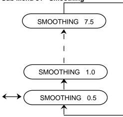
Rate is calculated and the rate display is updated every 0.5 seconds. Wen rate smoothing is selected to be greater than 0.5 seconds, the most recent rate calculation is averaged with the previous rate calculations that were made in the smoothing period. Use the up arrow key to select the amount of smoothing desired.
