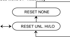
The Reset key can be programmed to unlatch the Ratemeter high and low alarms, or it can be programmed to have not effect on the alarms. Select the function of the reset key on the Ratemeter operation by pressing the up arrow key. The Reset key can be programmed for additional functions on the Totalizer operation. A chart is shown on page 15 to provide a convenient means of recording the tasks of the Reset key.
