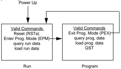
The third control command, reset, does not change the control's mode of operation, but merely performs a reset and/or unlatch function while leaving the control in the run mode. the Rest control command is suffixed by one digit (a) which allows for secondary functions to occur along
