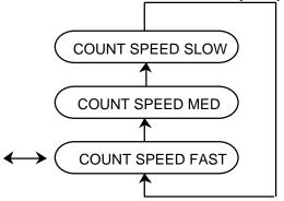
The maximum count input speed is selected in this menu. Use the up arrow key to select from FAST - 7.5 kHz max. MED - 400 Hz max.
