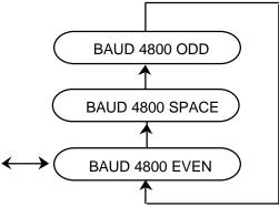
The baud rate and parity are set in this menu. Enter a baud rate of 300, 600, 1200, 2400, 4800, 9600 or 19200 by using the CLR, NUMBER and ENT keys. Enter EVEN, ODD or SPACE parity by using the up arrow key.
