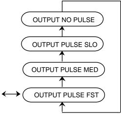
The totalizer pulse output transistor can be programmed for fast, medium, or slow pulse widths. It can also be programmed to not output pulses.
