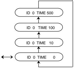
The unit identification number is set in this menu. Each unit on the communication bus must have a unique identifying number, 1 through 255. Enter the units ID by using the CLR, NUMBER and ENT keys. The length of time before the control response to communication requests can set to accommodate various types of computer equipment. Delay times of 0, 10, 100 and 500 milliseconds can be selected by using the up arrow key.
