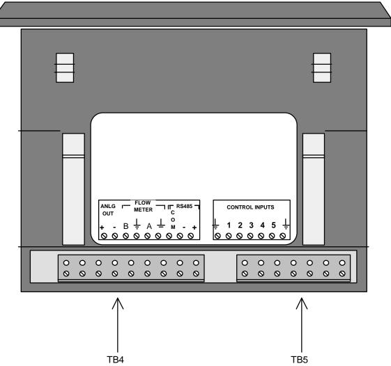
TB4 ANALOG OUTPUT( EA230-10), FLOWMETER INPUT, COMMUNICATIONS OUTPUT
