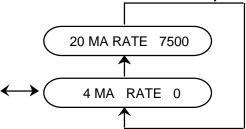
The rate output range is programmed at both the 4 mA and 20 mA points. This permit analog rate indications from 0 to full scale of the digitally displayed Rate or to select a portion of the Rate range. Use the up arrow key to select the 4 mA setpoints and then use the CLR, NUMBER and ENT keys to enter a Rate Value at each setpoint.
