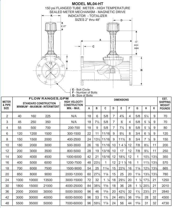
Standard construction will be supplied for all main line meters unless special flow range, materials, or construction are required. \* Minimum will be affected by Propeller Material and Extension Length.
